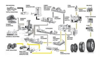
Figure 3. the industrial process for creating a tyre is very complex and articulated. It consists of about 16 different phases.
