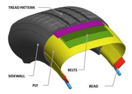
Figure 4. A tyre section schematization with main tyre components.
